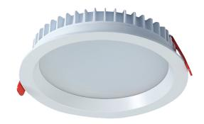
The Atlas Deep is a 140mm diameter low void downlight which uses a Samsung LED engine. The Atlas Deep has a 10mm recessed bezel feature for anti-glare cutoff. The heatsink is constructed from die-cast aluminium complete with aluminium bezel and reflector. The heatsink features spring arms which allows the downlight to be installed with ease.
