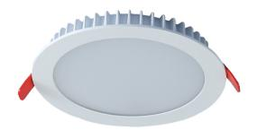
The Atlas Mini is a 104mm diameter low void downlight which uses a Samsung LED engine. The heatsink is constructed from die-cast aluminium complete with aluminium bezel and reflector. The heatsink features spring arms which allows the downlight to be installed with ease.
