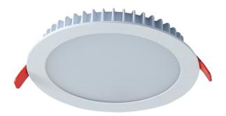
The Atlas is a 140mm diameter low void downlight which uses a Samsung LED engine. The heatsink is constructed from die-cast aluminium complete with aluminium bezel and reflector. The heatsink features spring arms which allows the downlight to be installed with ease.
