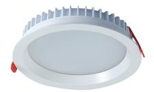
The Atlas Deep Mini is a 104mm diameter low void downlight which uses a Samsung LED engine. The Atlas Deep has a 10mm recessed bezel feature for anti-glare cutoff. The heatsink is constructed from die-cast aluminium complete with aluminium bezel and reflector. The heatsink features spring arms which allows the downlight to be installed with ease.
