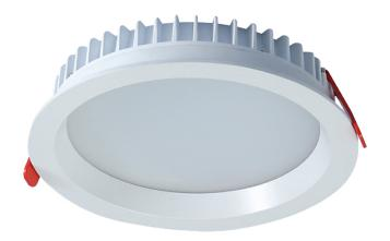
The Atlas Deep Max is a 180mm diameter low void downlight which uses a Samsung LED engine. The Atlas Deep has a 10mm recessed bezel feature for anti-glare cutoff. The heatsink is constructed from die-cast aluminium complete with aluminium bezel and reflector. The heatsink features spring arms which allows the downlight to be installed with ease.
