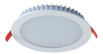
The Atlas Max is a 180mm diameter low void downlight which uses a Samsung LED engine. The heatsink is constructed from die-cast aluminium complete with aluminium bezel and reflector. The heatsink features spring arms which allows the downlight to be installed with ease.
